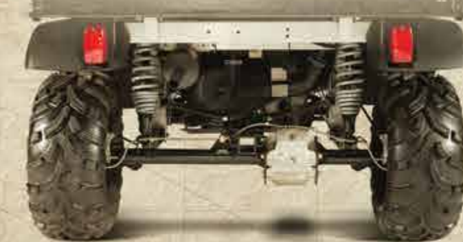
XRT1550 with heavy-duty, automotive 4-link suspension for up to 3/4-ton vehicle rated capacity
